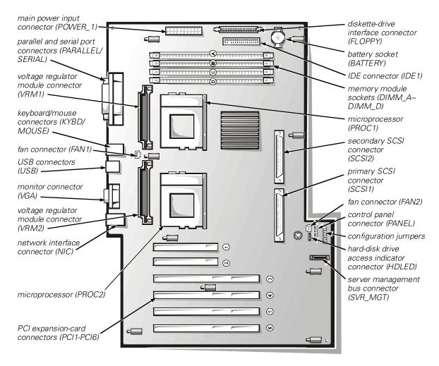
Figure 8-1. System Board Features
